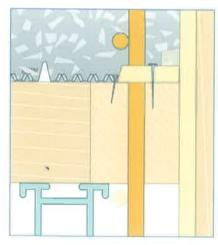
Ensure the cut edge is supported by timber or additional steel bar
